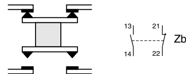
The 2 moving contacts are electrically separated
