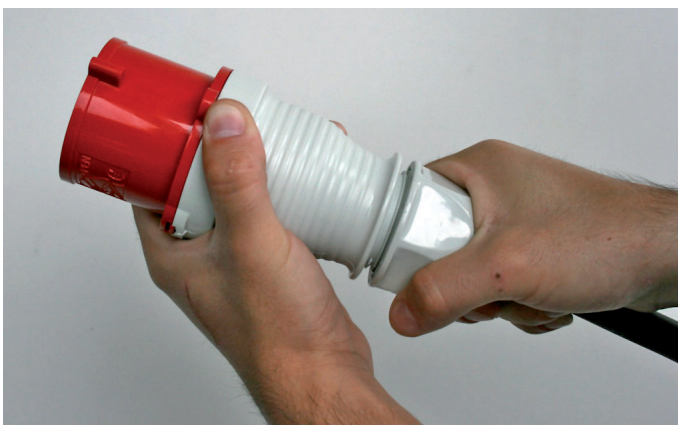
5. Finally tighten the cable gland (torque at least 4 Nm) - ready.
