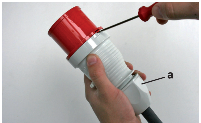
6. To disassemble first unscrew the cable gland (a). Then press a screwdriver, blade width 3,0 mm, deeply into the opening slot of the back part. Turn screwdriver clockwise to unlock the parts again.
