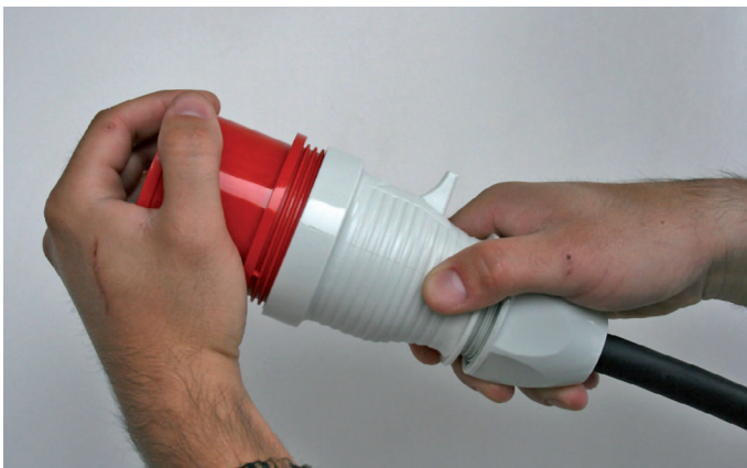
3. Adjust the back part on the thread of the front part and ...
