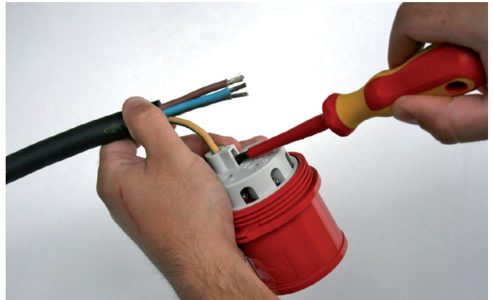
2. Connect all conductors according to the cover plate markings, using a screwdriver PZ1.
